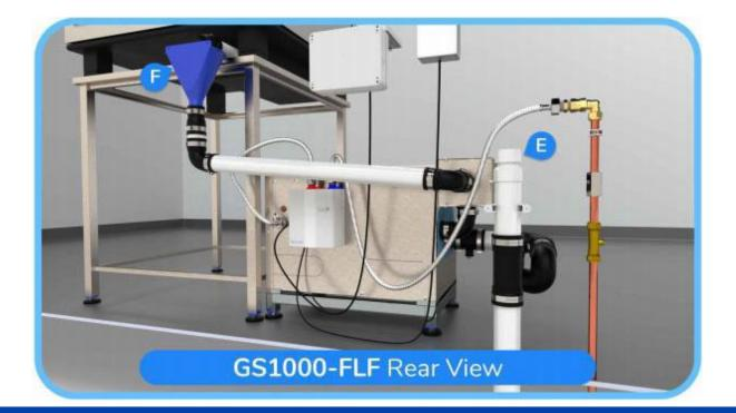
Pipe work must be  $42mm(1 \frac{1}{2})$  pipe work that is well supported and having a fall of at least 1 in 40.
